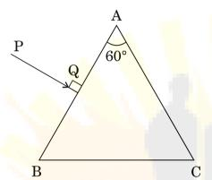
A ray PQ is incident normally on the face AB of a triangular prism of refracting angle of  $60^{\circ}$ , made of a transparent material of refractive index  $2/\sqrt{3}$ , as shown in the figure. Trace the path of the ray as it passes through the prism. Also calculate the angle of emergence and angle of deviation.
